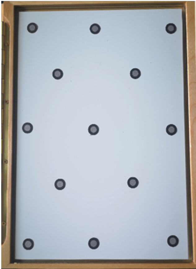
Figure 2 - 3D Handyscan calibration device with sample targets.
